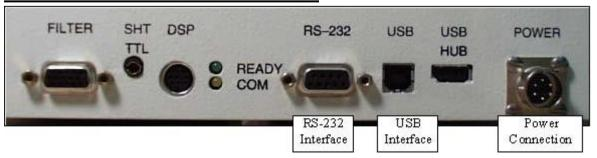
Figure 6. Details of the RS-232, USB, and Power Connections on the SP-2300i
